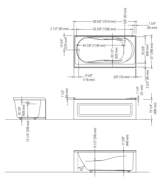
$<sup>\</sup>star$ A bathtub fitted with back jets can cause the pump to protrude by approximately 3" from the overall dimension.
