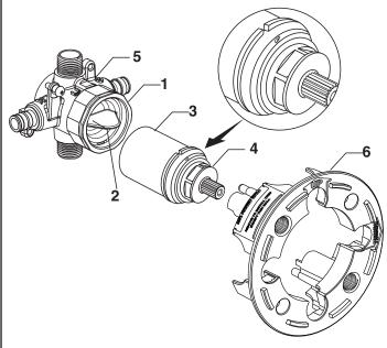
NOTE: Specified tightening torque of BONNET NUT (1) is critical to assure sealing function.
