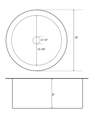
Dimensions of fixture are nominal and may vary within the range of tolerances established.
