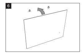
Install the mirror making sure the wall hangers are perfectly attached to the mirror back frame channel
