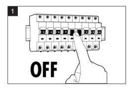
Disconnect electrical power from the main switchboard
