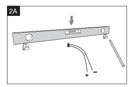
Secure the rest of the hangers using a level
