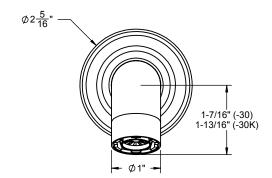
THROUGH-HOLE SPECIFICATIONS RECOMENDED **MAX** SPOUT: Ø1" Ø 1-1/4" Ø1-9/16"
