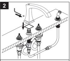
Place the spout washer under the spout and install spout on spout nipple-diverter assembly. Be sure the spout is firmly resting on the deck. Secure the spout with the setscrew.
