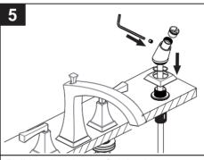
Pull black nylon or finished hose through the hand shower nipple bracket. Slide the hand shower "O" ring, bracket and hose guide over the hose. Secure the assembly with the setscrew. Note, make sure the hose does not slip under the deck.
