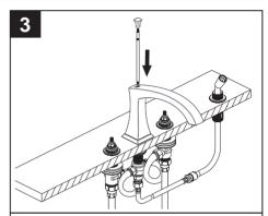
Insert diverter knob and rod assembly into the spout and thread the assembly onto the diverter rod in the spout diverter assembly. Pull the diverter rod and knob up and down to test the connection.
