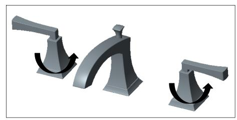
1. Hold the handle escutcheon and turn it counterclockwise to remove
