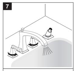
Make sure the diverter knob is in the down position. Turn the faucet handles on full for one minute to flush debris.
