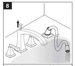
Leaving the water on, pull the hose to its farthest extension and point it into the tub. Pull the diverter knob to its top position. Flush the debris fro one minute. Turn off the valves.
