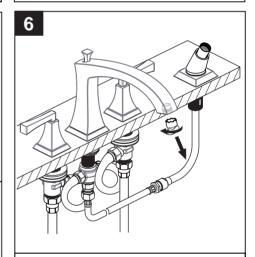
Remove the aerator with the supplied key. Turn the water supply on.
