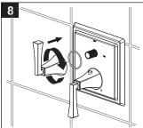
Set the volume control handle and escutcheon at 12 o'clock and place on the top stem and nipple. Rotate the escutcheon clockwise to secure the assembly to the plate.
