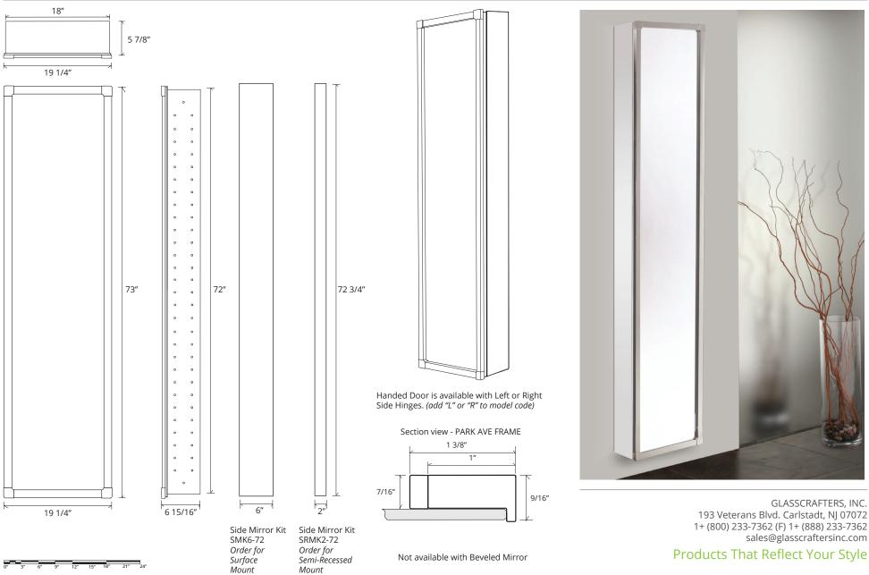
SPECIFICATIONSRoughing-in Opening18 3/8" x 72 1/8"Overall Dimensions19 1/4" x 73"
