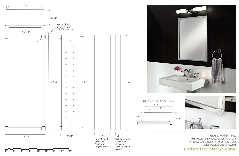
SPECIFICATIONSRoughing-in Opening14 3/8" x 35 3/8"Overall Dimensions15 1/4" x 36 1/4"
