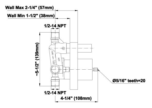
The measurements shown are for reference only. Products and specifications shown are subject to change without notice. Revised 06/2014. www.graff-faucets.com | phone: 800-954-4723 SHOWER Pressure Balancing Valve Trim with Handle & Diverter G-7095-C16S-T
