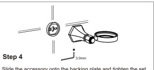
Slide the accessory onto the backing plate and tighten the set screw using Allen key provided.
