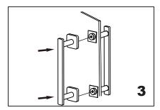
Add the handle B end caps on the fixing brackets, make sure the set screws holes in the bottom.
