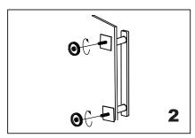
Screw in the fixing brackets into the handle bolts.
