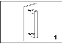
Install the handle A (bolt) through the glass holes, make sure the rubber gaskets are between handle&glass.
