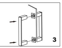
Add the handle B end caps on the fixing brackets, make sure the set screws holes in the bottom.
