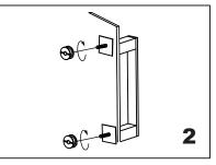
Screw in the fixing brackets into the handle bolts.
