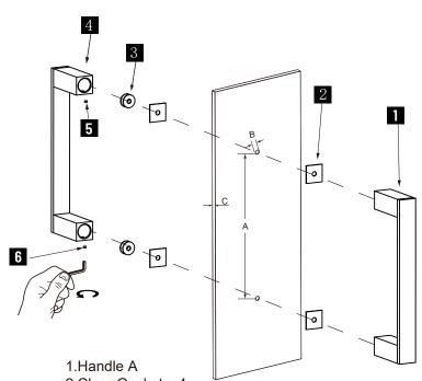
2.Clear Gasket x 4 3. Fixing Bracket x 2 4.Handle B 5.Set Screw M5 x 2 6.Allen Key 2.5mm x 1
