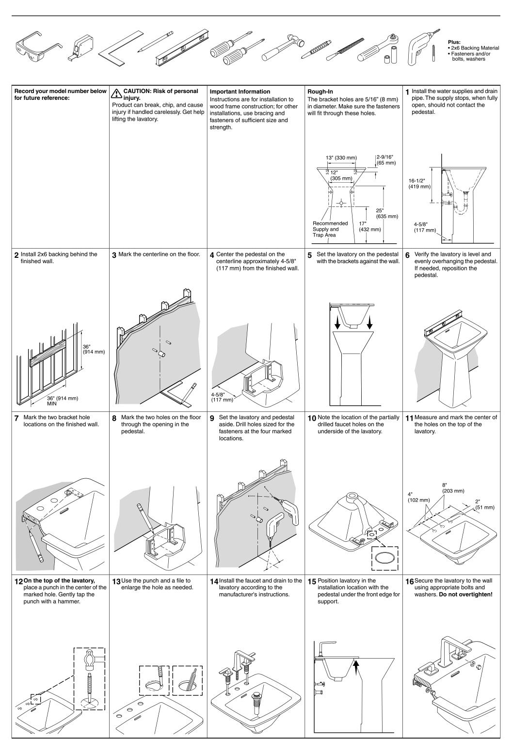
17 Move the pedestal under the lavatory, aligning the bracket holes with the holes in the floor.
