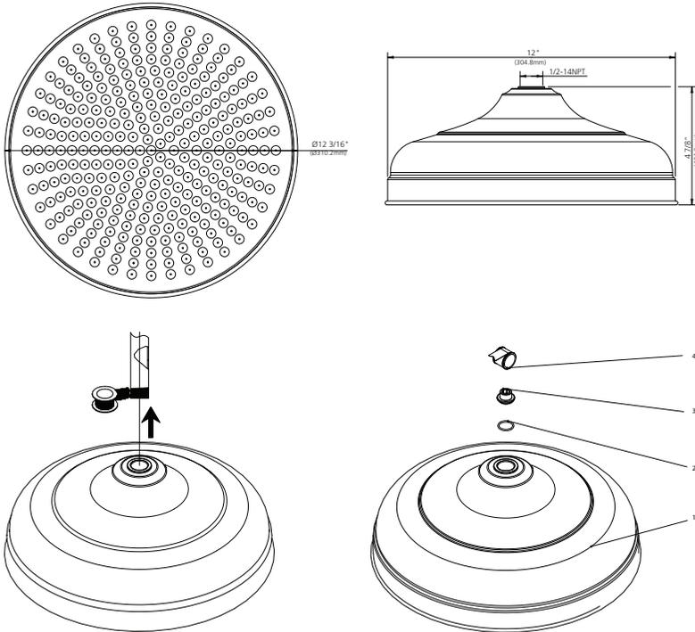
Wrap Teflon tape around the threads of the connecting pipe in a clockwise direction. Thread the shower head on the tape of the pipe and hand tighten as tight as possible.
