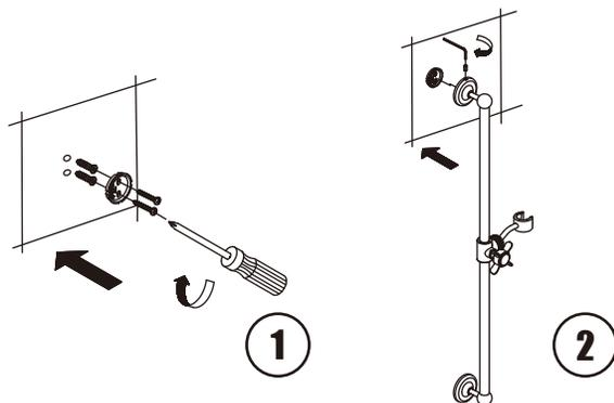
**1** Position the mounting bracket on the wall where required. Mark the location of mounting screws. Drill holes in the wall to fit the anchors. Tap the plastic anchor into the hole with a hammer. Position the mounting bracket to be mounted on the wall, then thread the fixing screws through the mounting hole into the plastic anchor. Tip: install one post, then assemble slide bar to confirm hole position of second post before drilling.
