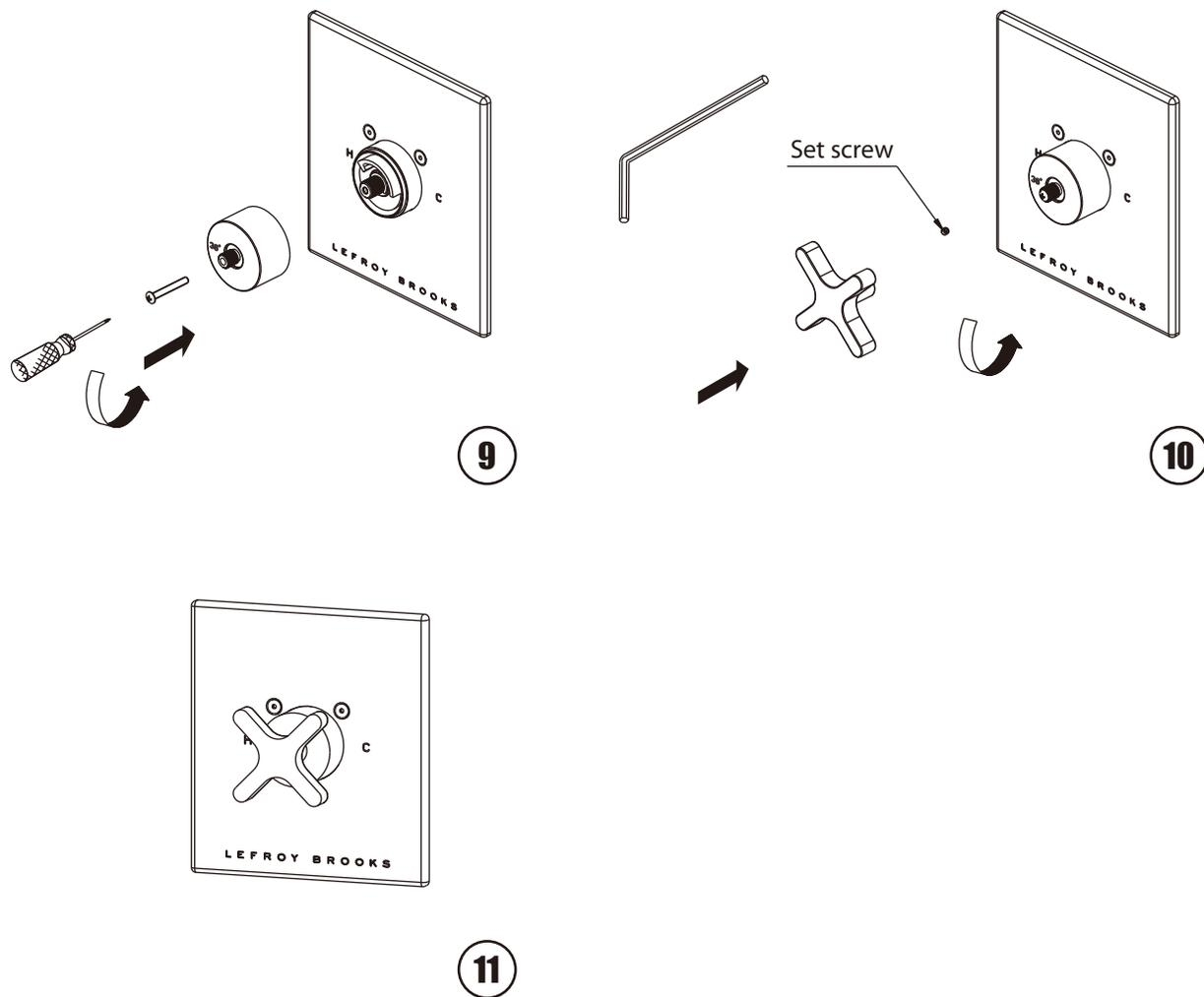
**9** Fix the canopy with screw. When it is fixed, the temperature-limit-button is at horizontal position.
