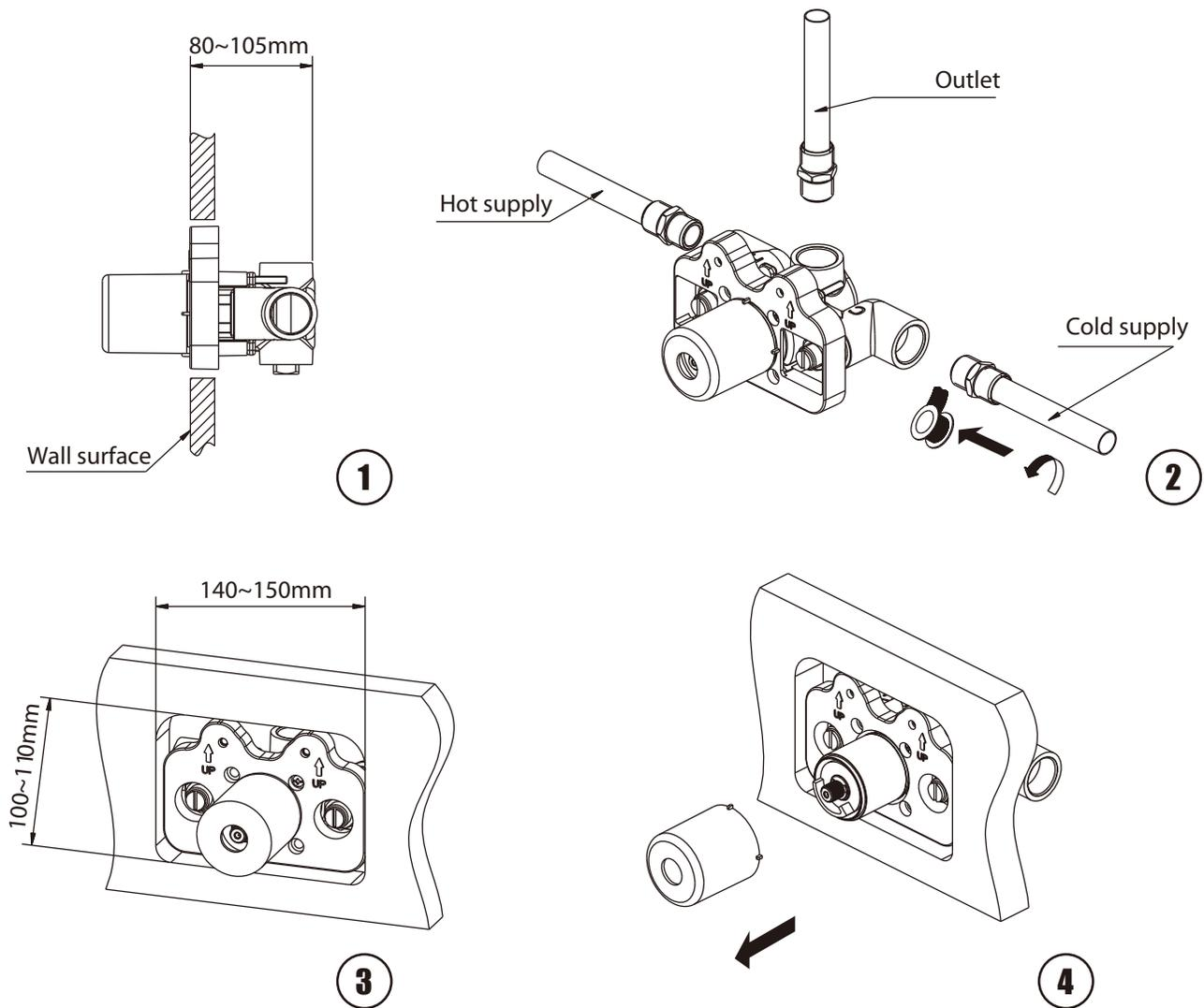
**1** Before installing the valve into the wall, please note that a distance between 80mm~105mm from the wall surface to the rear of the valve should be left so that can fit the trim kit further.
