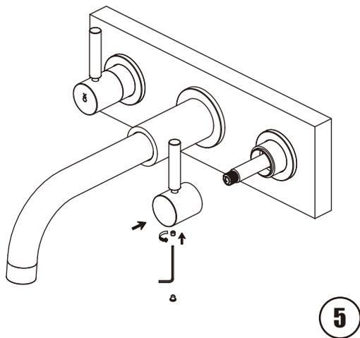
**5** Install and fix handle with set screw.
