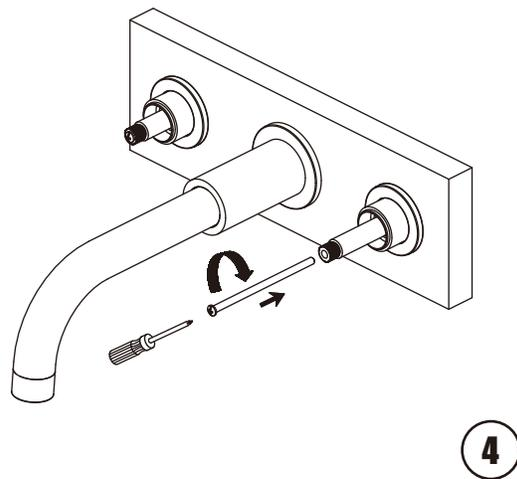
**4** Install stem extension to the rough and fix securely with screw.
