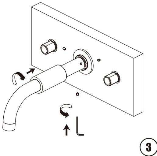
**3** Install the spout and then fix the central canopy onto the spout securely with the grub screws.
