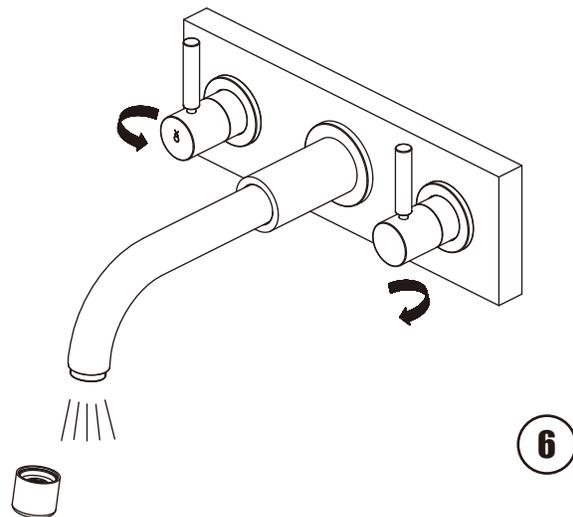
**6** After installing the faucet, remove aerator and open the hot and cold supplies. Check for leaks. Turn on the faucet handle for one minute to flush debris from the faucet. Turn off the handle and re-assemble the aerator.
