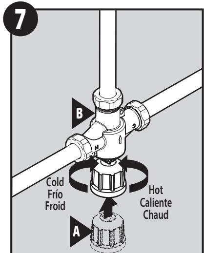
To adjust temperature: Align triangle on top of Adjustment Cap (A) with triangle on top of Valve Body (B). Twist counter clockwise for hot or clockwise for cold.
