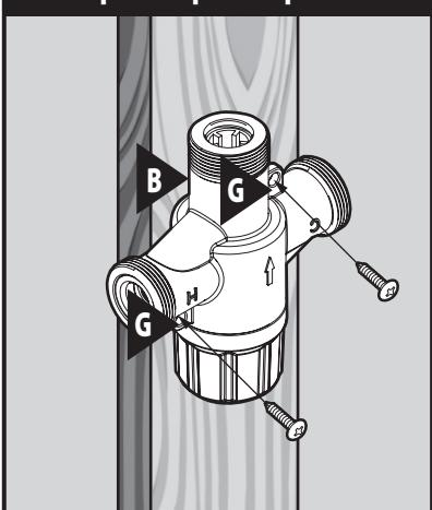
To secure valve (B) for easier installation, insert screws through mounting tabs (G) and mount to 2x4 or other available surface.
