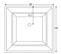
As vessel, installs on top of counter.
