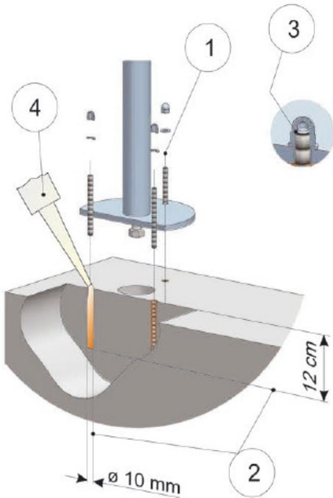
1. Place the shower column into position and trace the 3 fixation holes. Remove the column.
