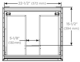
Top view for plumbing and sink clearance
