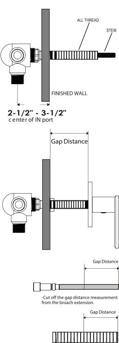
4. Reinsert the nut, washer and handle onto the stem.
