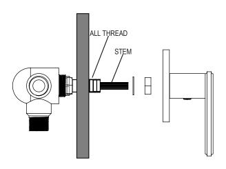
5. Using the Allen Key provided, tighten the handle set screw firmly.
